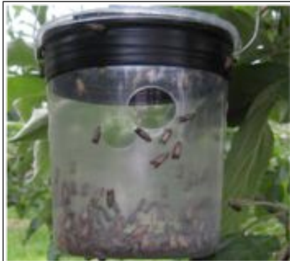
Figure 4. SIR moth release device used in research trials. Moth are dumped into a release cup and allowed to exit through holes in the sides of the cup.
